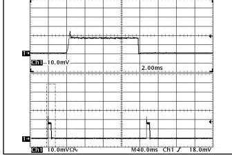
Figure 18: Load current (10A/div) as a function of time when the converter attempts to turn on into a 10 m $\Omega$  short circuit. Top trace (2.0ms/div) is an expansion of the on-time portion of the bottom trace.
