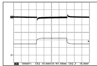
Figure 11: Output voltage response to step-change in load current (50%-75%-50% of Iout(max);  $dI/dt = 0.1A/\mu s$ ). Load cap:  $10\mu F$ ,  $100 \text{ m}\Omega$  ESR tantalum capacitor and 1µF ceramic capacitor. Ch 1: Vout (100mV/div), Ch 2: Iout (5A/div).
