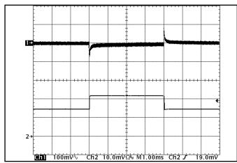
Figure 12: Output voltage response to step-change in load current (50%-75%-50% of Iout(max):  $dI/dt = 5A/\mu s$ ). Load cap: 470 $\mu F$ , 30 m $\Omega$  ESR tantalum capacitor and 1µF ceramic cap. Ch 1: Vout (100mV/div), Ch 2: Iout (5A/div).
