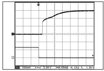
Figure 10: Turn-on transient at zero load (4 ms/div).
