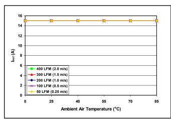
Figure 7: Maximum output power-derating curves vs. ambient air temperature for airflow rates of 50 LFM through 400 LFM with air flowing from input to output (nominal input voltage).
