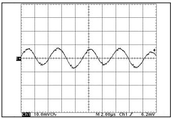
Figure 15: Input Reflected Ripple Current,  $i_s$ , through a 10  $\mu$ H source inductor at nominal input voltage and rated load current (5 mA/div). See Figure 13.
