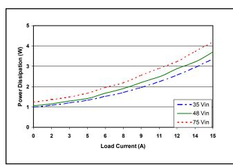
Figure 3: Power dissipation at nominal output voltage vs. load current for minimum, nominal, and maximum input voltage at 25°C.
