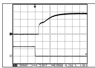
Figure 9: Turn-on transient at full load (resistive load) (4 ms/div). Input voltage pre-applied. Ch 1: Vout (500mV/div). Ch 2: ON/OFF input (5V/div)
