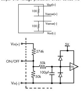
Figure B: Internal ON/OFF pin circuitry
