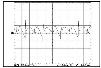
Figure 16: Output Voltage Ripple at nominal input voltage and rated load current (20 mV/div). Load capacitance: 1µF ceramic capacitor and  $10\mu F$  tantalum capacitor. Bandwidth: 20 MHz. See Figure 13.
